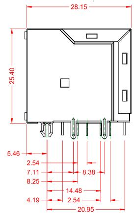
RJ45, 6 PORTS, RIGHT ANGLE PCB MOUNT
