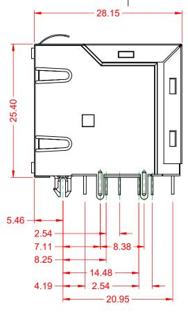
RJ45, 4 PORTS, RIGHT ANGLE PCB MOUNT
