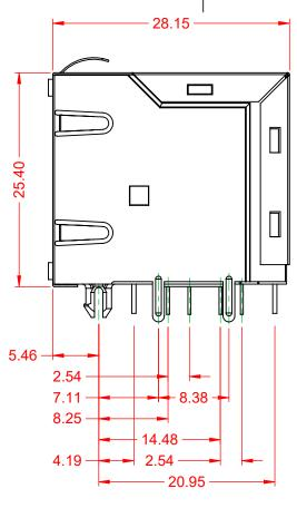
RJ45, 4 PORTS, RIGHT ANGLE PCB MOUNT
